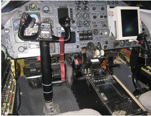
The L1 was evaluated by the pilot in the right seat using a joystick. The left seat, with the conventional Learjet controls, is for the safety pilot. Credit: Guy Norris/AW&ST
