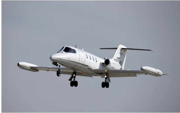
Tests of the controller in Calspan's variable-stability Learjet included dealing with roll-coupled yaw while simulating a lifting body and high adverse aileron yaw while replicating an F-100 Super Saber. Credit: Calspan
